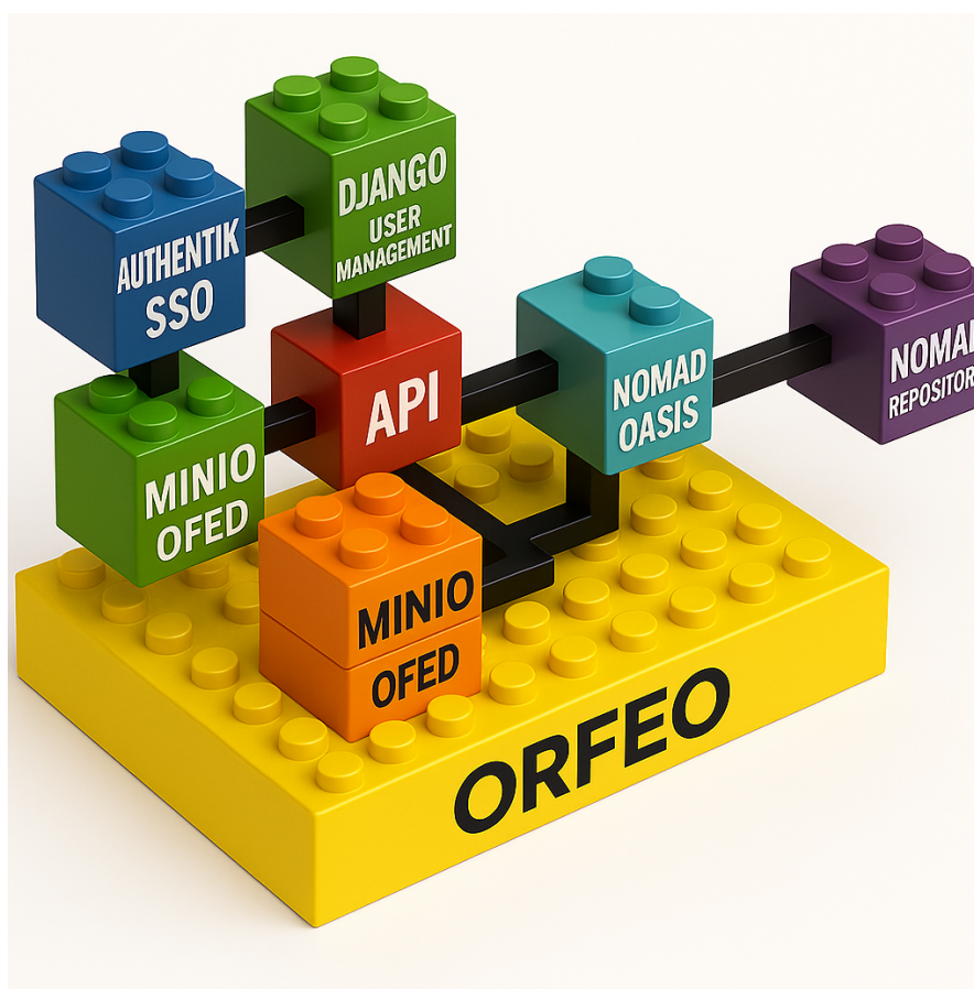
Figure 3.2: System architecture overview: User access and authentication via Authentik; data transfer to MinIO; metadata indexing in PostgreSQL; registration in ORFEO; publication to NOMAD Oasis and external repositories.
